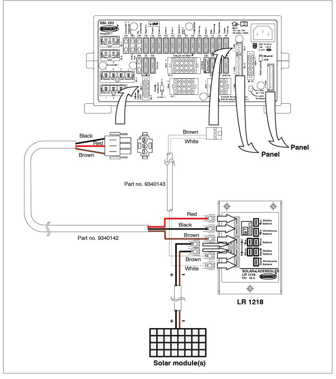
Fig. 4 LR1218 to Schaudt EBL with 3-pin solar regulator connector (e.g. EBL 223) Solar module(s) and their connector cables are not included in the delivery.
