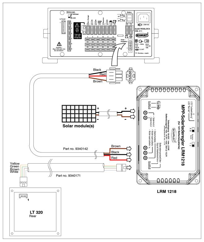
6.2 LRM 1218 and Schaudt EBLs with 3-pin solar connector
