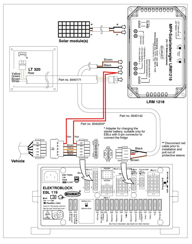
6.3 LRM 1218 and Schaudt EBLs with 2-pin solar connector, and adapter for the starter battery
