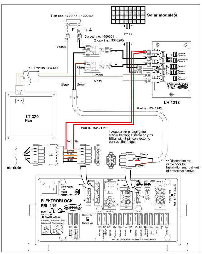
5.3 LR 1218 and Schaudt EBLs with 2-pin solar connector, and adapter for the starter battery
