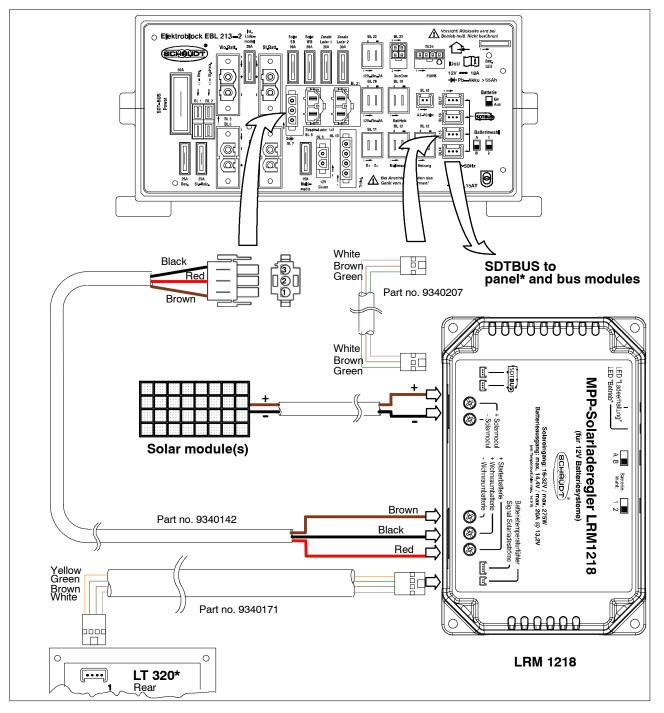
Fig. 11 LRM1218 to Schaudt bus-compatible EBL and additional display via LT320
