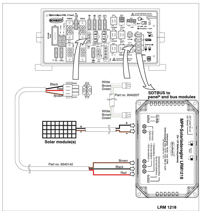
Set 9990314 (LRM 1218 with connector material) is required.
