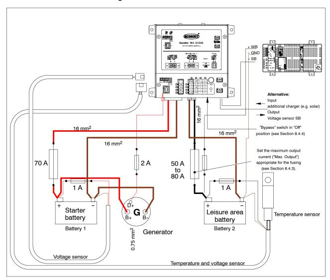
Fig. 9 Vehicles without Schaudt EBL - direct connection to batteries
