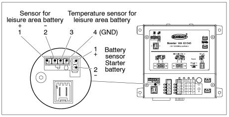
Fig. 10 Temperature sensor: Connection
