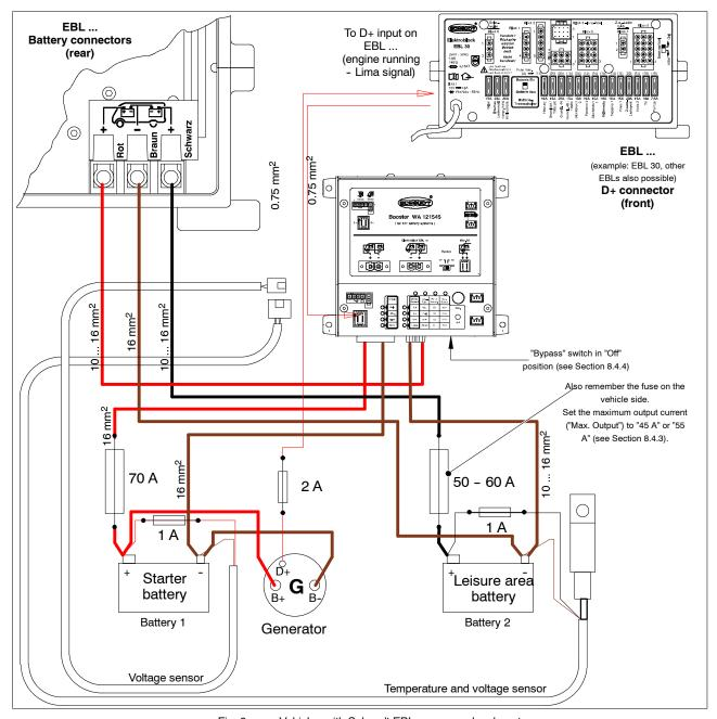
Fig. 6 Vehicles with Schaudt EBL ... - ground on booster
