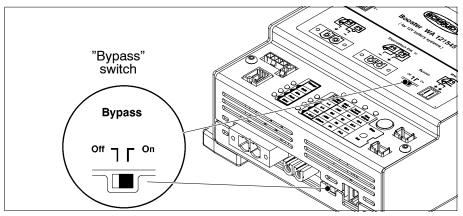
Fig. 13 "Bypass" sliding switch
